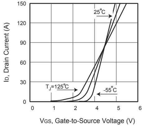
**Figure 2. Transfer Characteristics**
