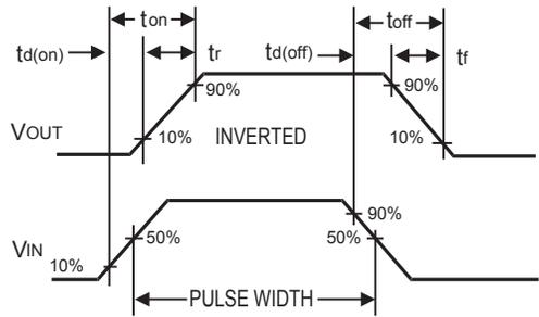
Figure 10. Switching Waveforms
