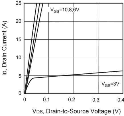
**Figure 1. Output Characteristics**
